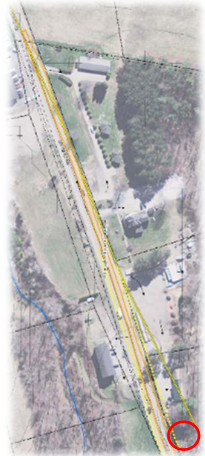
Figure 17: Drainage area for the Rte_5_Erosion_a gully. Gully location indicated in red below.
