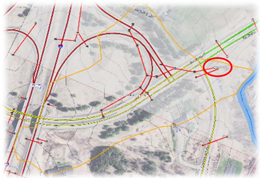
Figure 7: ORL_006 drainage area and infiltration basin site on VTrans-owned land in Orleans Village.
