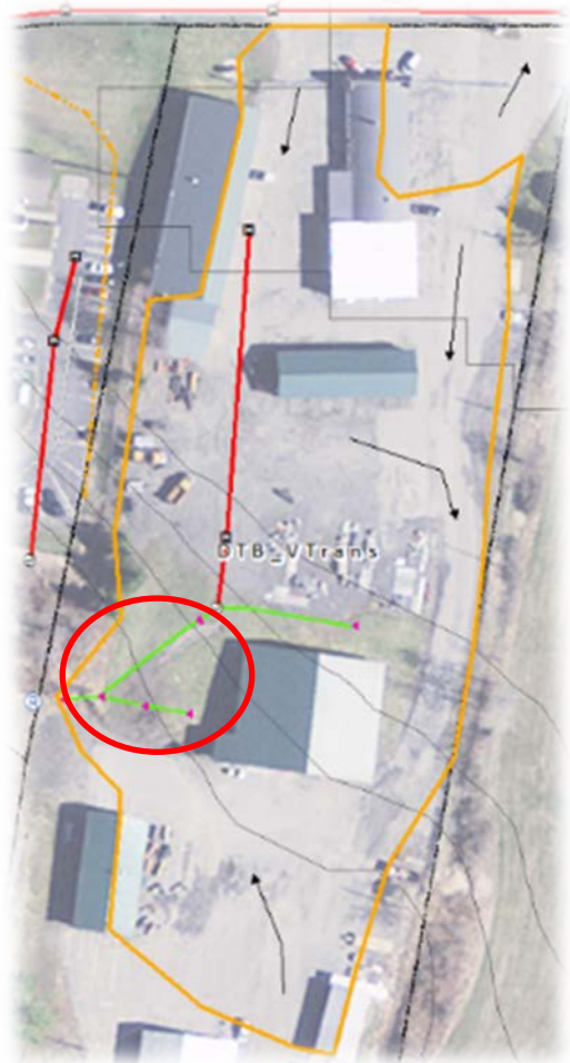
Figure 16: DTB_VTrans drainage area and potential BMP site.
