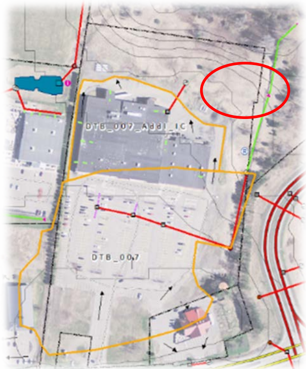
Figure 10: DTB_007 drainage area and approximate BMP location (Shaw’s Shopping Center).
