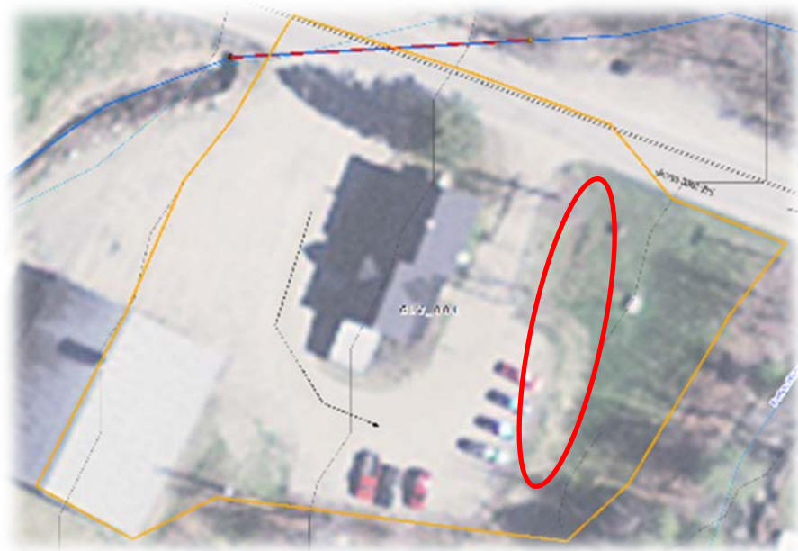
Figure 15: GLV_001 drainage area and potential BMP location.
